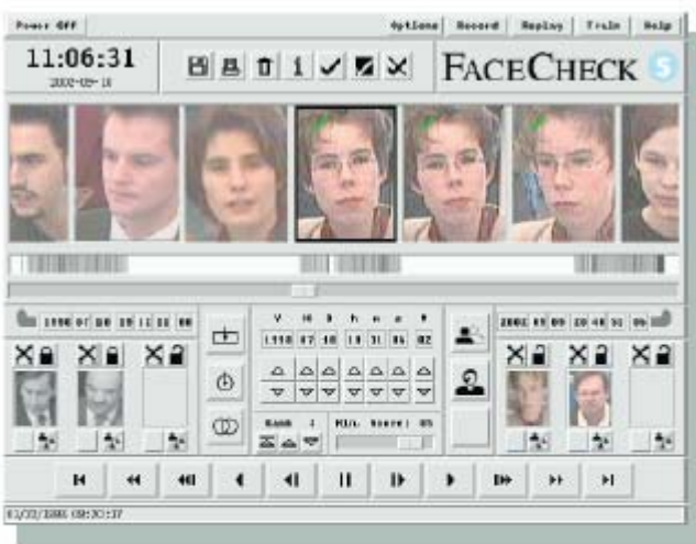
In search mode, the user can define image groups and search criteria for face identification. Automatic functions for image pattern recognition can also be used to search the image database.
