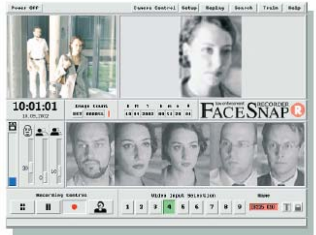
In recording mode, the FACE SNAP RECORDER screen simultaneously shows the live camera shot and the latest sequence of captured facial images.
