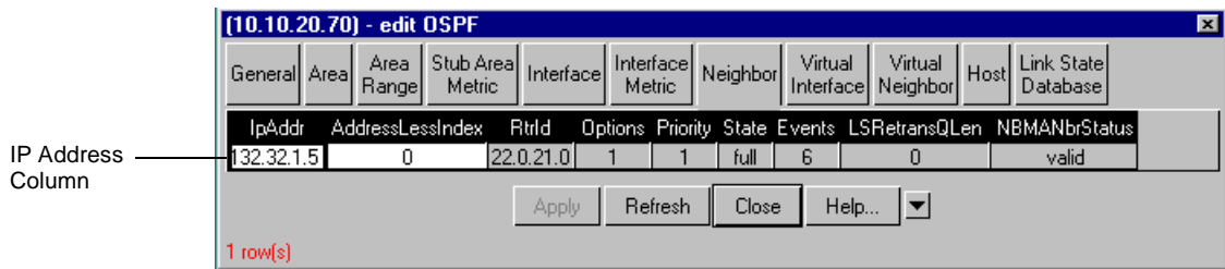
Figure 11-16. Switch 1 Neighbor Window
